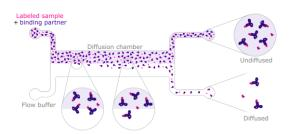
Fluorescently labelled proteins enter the microfluidic diffusion chamber together with an auxiliary fluid, in two parallel laminar streams. The rate of diffusion of proteins from one stream to the other depends on the protein molecular size (top)
